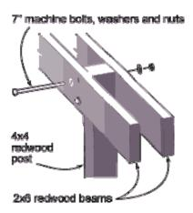
Two 12-foot-long 2x6 beams are attached to each set of posts, one on each side and extending 18 inches outward from the centre line of the posts. Nail or screw the beams to position them even with the tops of the posts. Drill two 1/2" diameter holes through the double beams and posts. Secure with two 7-inch machine bolts.
