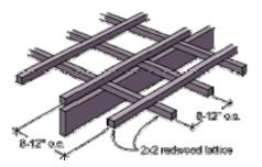
**Custom lattice** You can design and build your own lattice pattern to meet your shade requirements. Layout the 2x2s for the custom lattice and assemble with non-corrosive fasteners before securing to the rafters.
