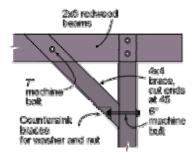
Cut the remaining 4x4s into four pieces, each 30 inches long and with a 45-degree angle on each end. Fasten the bottom of each brace with a 6-inch machine bolt and countersink the washer and nut. The top of the brace is sandwiched between the double beams and secured with a 7-inch machine bolt.
