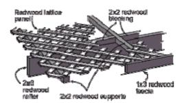
**Ready-made lattice** As an alternative to louvers, consider using ready-made redwood lattice that will provide moderate filtered sunlight in an interesting pattern. Use 2x2 redwood as sup-ports and blocking. Attach the preassembled 4x8 lattice panels to the 2x2s with 1-inch, non-corrosive fasteners. For a more finished look, frame the lattice all around with 1x3 redwood fascia.
