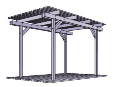
A simple weekend project, this shelter will shade an area of approximately 8 feet by 12 feet or 96 square feet. The basic plan can be modified by adding more posts, longer beams and additional louvers. If you decide to enlarge this project, keep in mind that the rafters should span no more than 6 feet.
