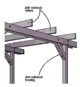
The 8-foot 2x6 rafters start over the posts and are spaced 18 inches o.c. Toenail each rafter with 8d nails on top of the beams extending 12 inches outward front and rear. Secure the rafters with two nails driven through each side of the rafters and into each of the double beams. Screws may also be used. In either case, Predrill to prevent splitting. Remove post bracing.
